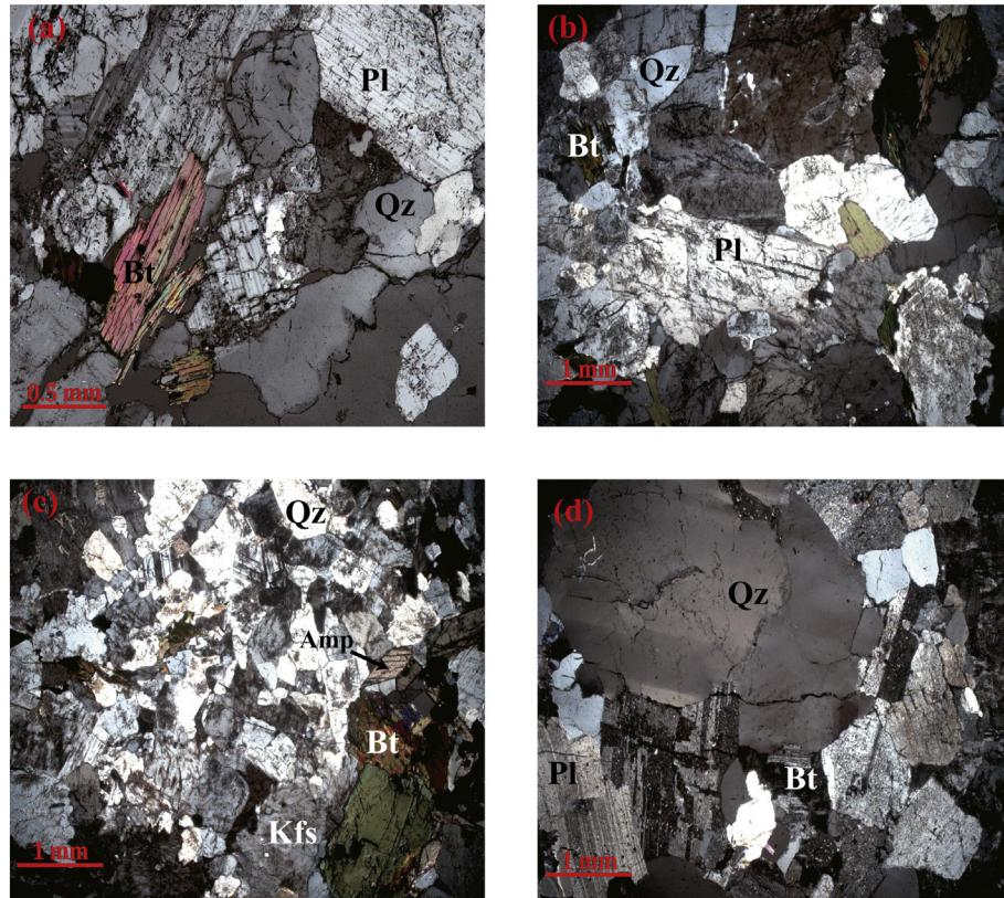
**Fig. 2.** Photomicrographs showing mineral assemblage of representative granitoids ((a) sample XX14-01, (b) sample WY14-07, (c) sample TTZ14-05, (d) sample CS14-01). The abbreviations are: Pl-plagioclase, Qz-quartz, Bt-biotite, Kfs-K-feldspar, Amp-amphibole.
