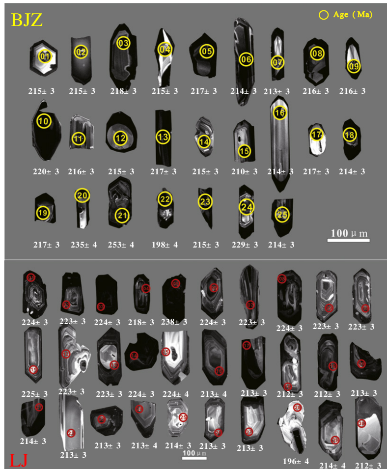
Cathodoluminescence (CL) images of representative zircons from the host granitoids of the BJZ and the LJ plutons. Spots for zircon U–Pb dating using LA–ICP–MS and ages derived from zircons are also shown.
