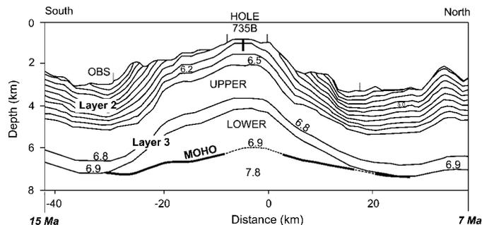
Figure 2. P-wave seismic velocity model for the Atlantis Bank and surrounding area on the north-south Line CAM 101 (Muller et al., 1997). The velocity contour interval is 0.3 km/s, and the OBS (ocean-bottom seismograph) locations are shown on the seafloor. The position of Hole 735B has been projected to the line from 1 km to the west.
